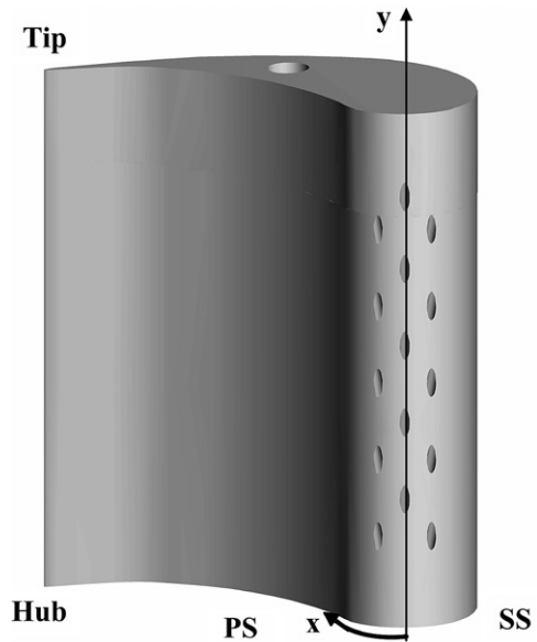
Fig. 6. Modified film cooling blade with three rows of radial-angle holes.
